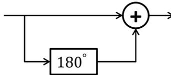
It is essential to realize that a good null can be achieved only if two conditions are met. First, the phase shift must be very close to  $180^\circ$ . Second, the amplitude of the original sinusoid must be equal to that of the inverted copy.
